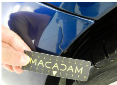
Holes and/or cracks in the bumper
